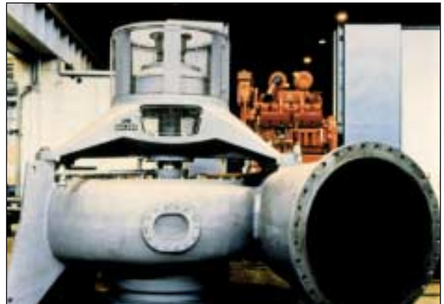
Pump sets. Couplings fitted between electric motors and pumps.
