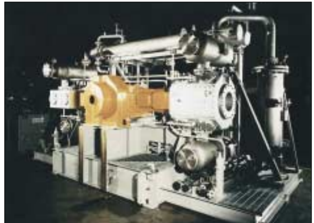
Compressor sets. Coupling fitted between electric motor and compressor units.
