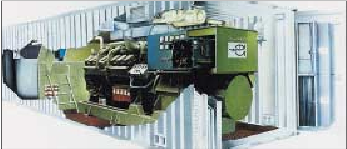
Mobile diesel generator sets. Coupling fitted between diesel engine and alternator.
