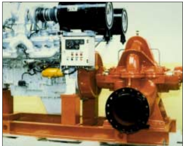
Pump sets. Coupling fitted between diesel engine and centrifugal pump.
